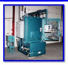
Make room for the super-duty cleaning machine – the PMW Model 812 Power Spray Washer. Many sizes and options available, including 36"-120" dia. turntable, 1,000-15,000 lb. capacity, 15-75 hp. pump motor, 24"-144" working height, fully insulated cabinet, 7-day timer, and much more
