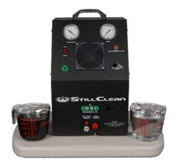
**Power requirements:** 110 volt, 5.4 Amps, 50/60 Hz **Compressed air:** 0.5 CFM @ 80 PSI minimum supply pressure **Clean solvent output:** Over 1 gallon per hour
