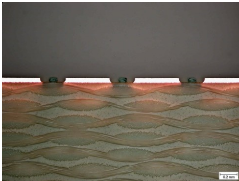
50 micron solder-dams (exposed using Olec ATH30)
